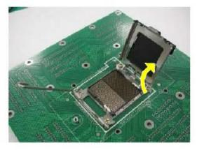
5. Locate the Pin 1 indicator of the package. Align the package with the socket and carefully insert the package into the socket with vertical motion only. Vertically check if the CPU is seated well in the socket housing. If not, take out the CPU, with vertical motion only, and repeat the above steps.
